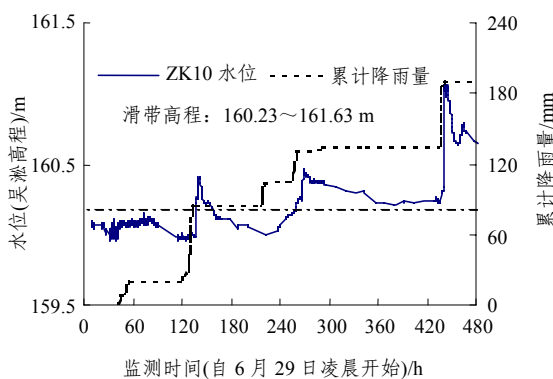
图 6 钻孔水位与降雨的关系 Fig.6 Water level in borehole vs. rainfall
