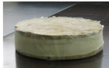
图 2 膨胀土不均匀收缩试验试样 Fig.2 The sample of expansive soil in uneven shrinkage test
