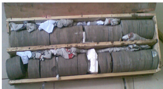
图 2 西部某油田硬脆性泥岩岩芯 Fig.2 Hard-brittle mudstone core of an oilfield in western China
