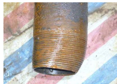
图4 套管接箍损坏 Fig.4 Casing coupling damage
