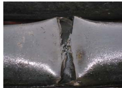
图3 造腔现场提出的断裂造腔外管 Fig.3 The fractured casing in-situ
