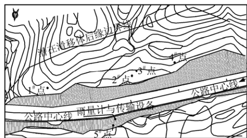
图9 仪器平面布置图 Fig.9 Plan layout of monitoring devices in the slope
