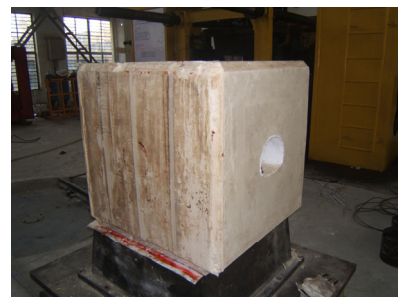
图 7 加长锚喷层试验后形态 Fig.7 Failure modality of lengthened bolt and jetting reinforcing tunnel
