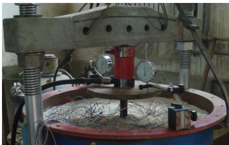
图1 模型箱与模型桩 Fig.1 Testing chamber and model pile
