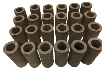
图 3 空心圆柱岩石试样 Fig.3 Rock specimen of hollow cylinder
