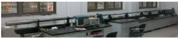
图 1 SHPB 实验装置 Fig.1 SHPB test equipment
