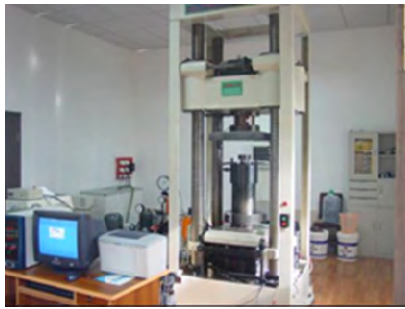
图1 XTR01 型高温高压岩石伺服试验机 Fig.1 XTR01 servo controlled rock mechanical test machine of high temperature and high pressure
