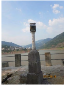
图 2 BGK-9060-01X 一体化水位监测站 Fig.2 Integrated water level monitoring station of BGK-9060-01X
