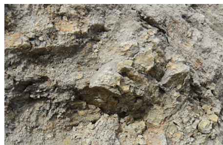
图 1 黄褐色膨胀性泥岩 Fig.1 Yellow-brown swelling mudstone
