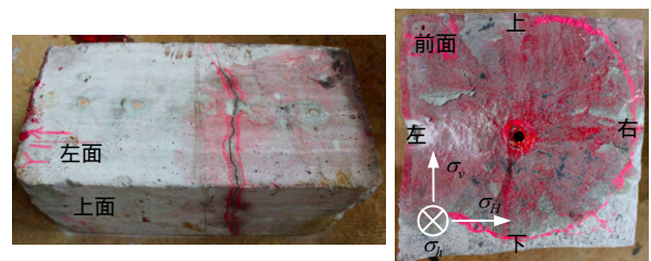
图 10 试样 N-2 典型水力裂缝形态 Fig.10 Typical geometry of hydraulic fracture of sample N-2
