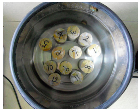
图3 置于真空饱和装置中的试样 Fig.3 Specimens in a vacuum saturation device
