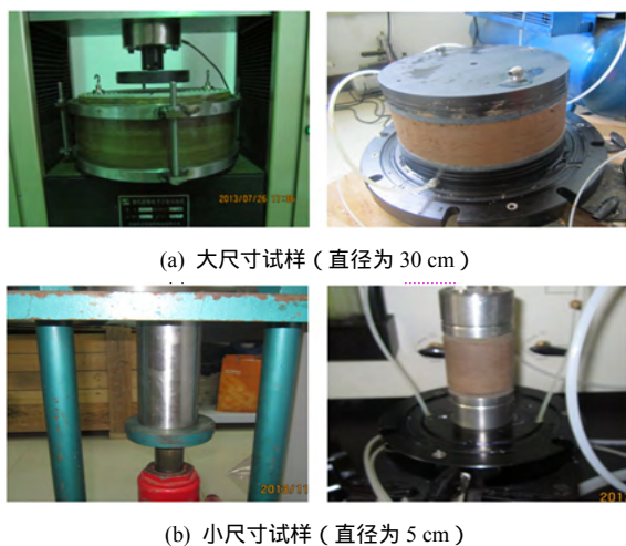
图1 试样制作与渗透试验过程 Fig.1 Process of specimen preparation and permeability testing
