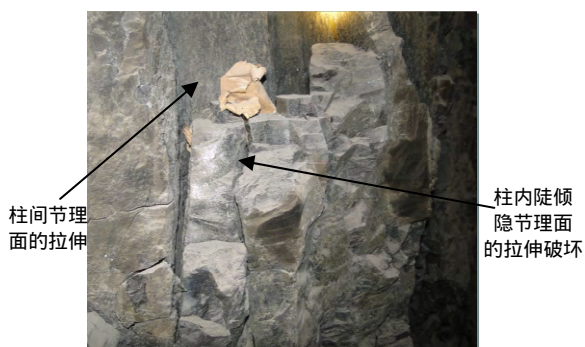
图 16 典型的柱状节理岩体表层破坏图 Fig.16 Typical joint slip at the surface of columnar jointed rock mass
