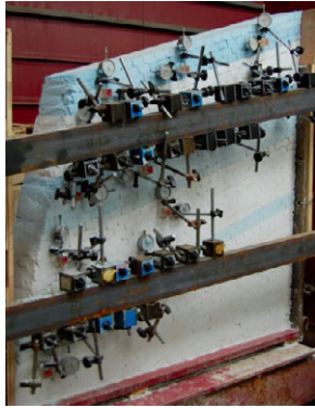
图3 百分表安装图 Fig.3 Dial gauge installation
