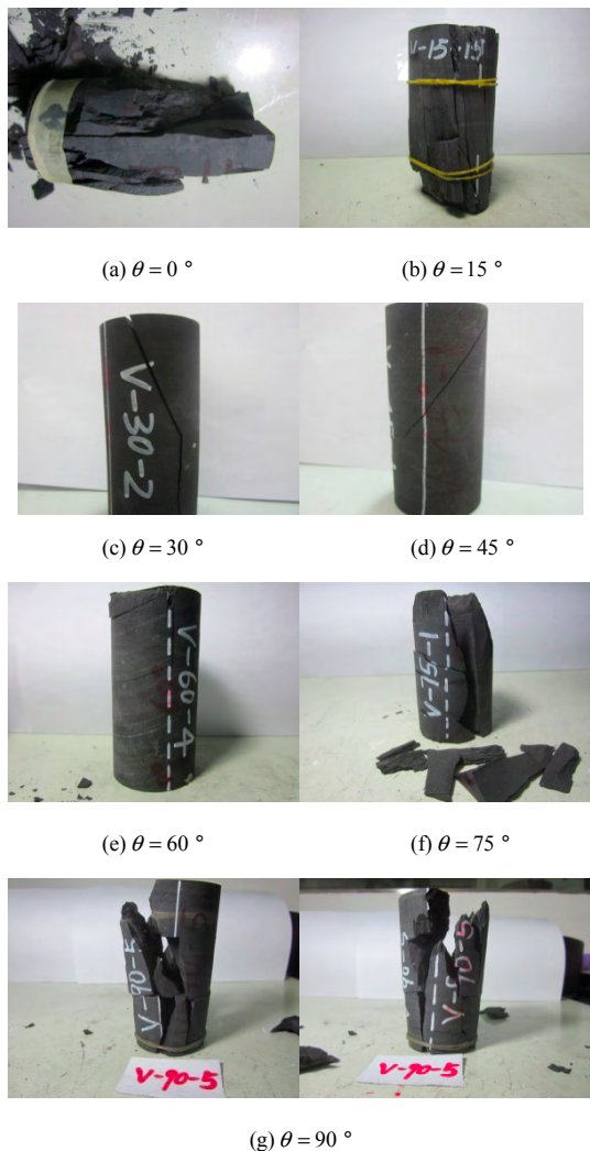
图 7 典型页岩试样破坏形态 Fig.7 Typical failure patterns of shale samples
