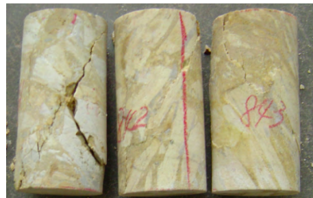
图 5 单轴压缩破坏的角砾岩裂纹特征 Fig.5 Cracks of breccia after uniaxial compressive test
