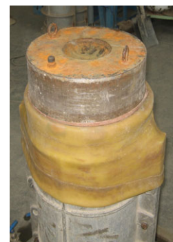
图 3 粗粒料三轴试验 Fig.3 Triaxial test for coarse grained materials
