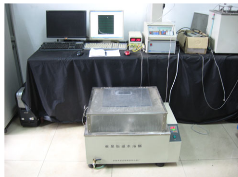
图 2 应力条件下原煤等温吸附试验装置照片 Fig.2 Photo of testing apparatus for measuring isothermal adsorption of coal under stress conditions
