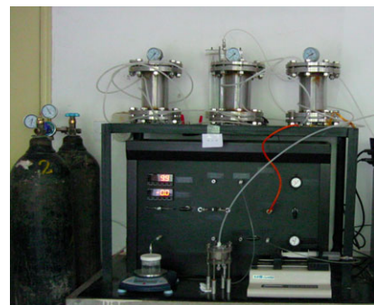
图 6 多步流动试验装置 Fig.6 Photo of multistep outflow experimental apparatus
