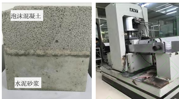
图 1 泡沫混凝土-水泥砂浆试样及 RMT-150C 伺服试验机 Fig.1 The foam concrete-cement mortar specimen and RMT-150C electro-hydraulic servo testing machine
