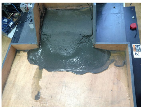
(c) Tailings expanding downstream
