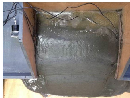
(b) Tailings mortar expanding at the toe of the tailings dam model
