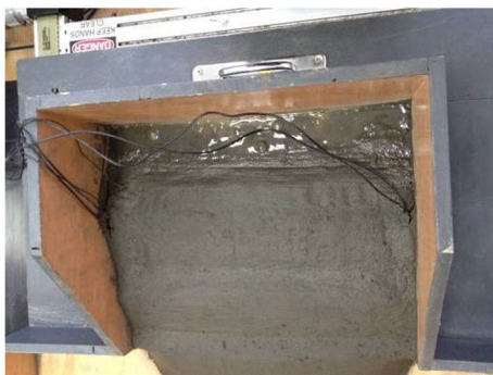
(a) Small amount of water being released from the dry beach
