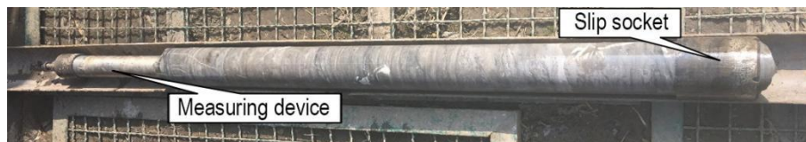
Figure 10. Recycling of borehole deformation measurement device and core after the test
