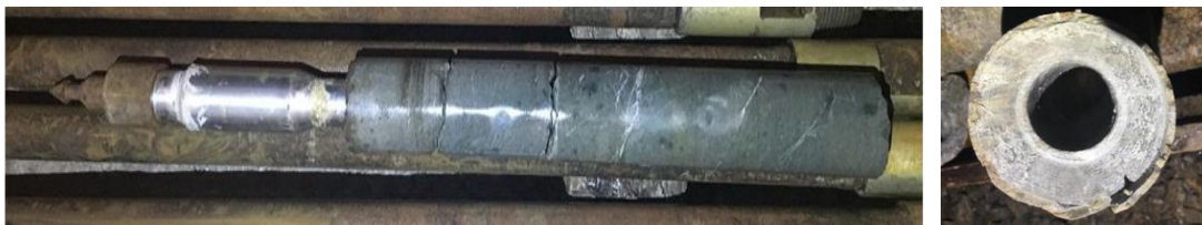
Figure 7. Annular core and borehole deformation measurement device.
