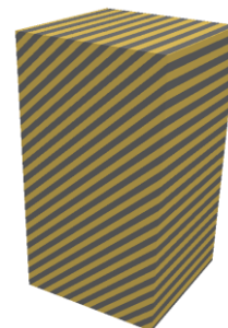
图10 含有一组贯通裂隙的离散元模型 Fig.10 Discrete element model with one penetrated joint set
