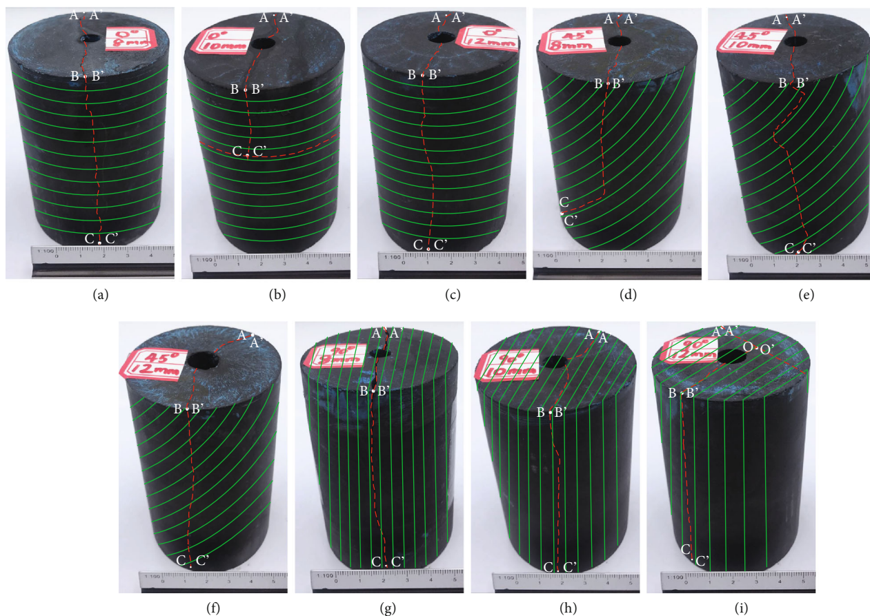
FIGURE 9: Macroscopic fracture morphology of HF created on the shale specimens.
