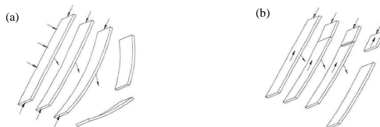
Figure 9. Failure mode of layered rock mass during tunnelling. (a: left-side arch; b: right-side wall).
