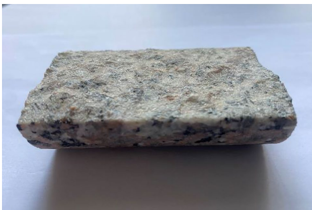
Fig. 6 A fracture surface with 50-mesh quartz sand
