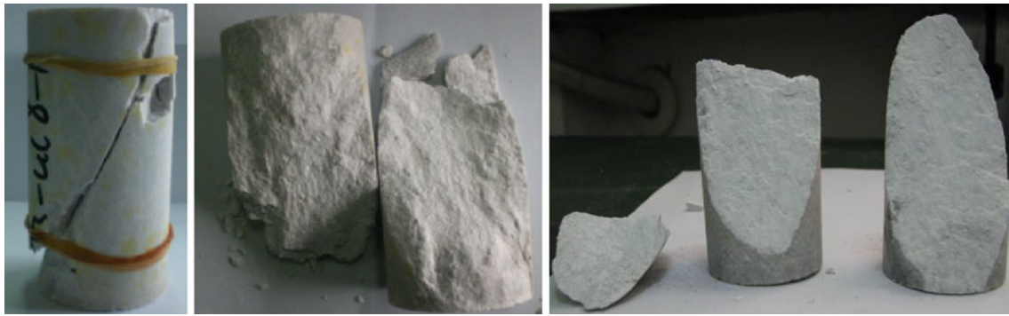
Fig. 9 Failure of marble under multi-step uniaxial compression creep testing
