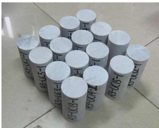
Fig. 3 Rock samples for time-dependent mechanical testing
