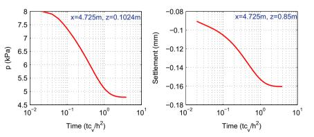
**Fig. 4.** Pore pressure dissipation in sand bed, and subsidence of breakwater in consolidation process. (Noted: *h* is the depth of seabed foundation, and *c<sub>v</sub>* is the consolidation coefficient of seabed soil.)
