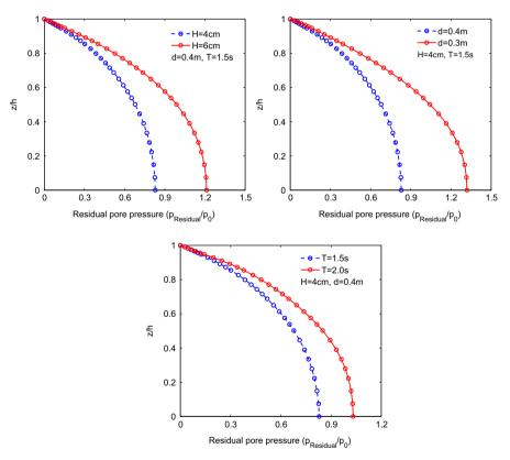
**Fig. 19.** Effect of wave characteristics on the wave-induced residual pore pressure in the loose sand bed at t/T = 20 ( $k = 1.0 \times 10^{-5}$  m/s,  $S_r = 98\%$ ).
