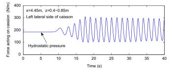
Fig. 9. Wave-induced impact force acting on the left lateral side of caisson.
