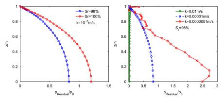
Fig. 20. Effect of soil properties on the wave-induced residual pore pressure in the loose sand bed at t/T = 20 (H = 6 cm, d = 40 cm, T = 1.5 s).
