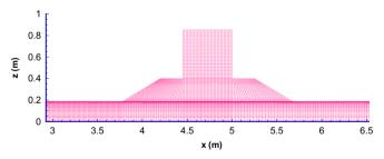
Fig. 3. FEM mesh used in computation for sandy bed and composite breakwater.
