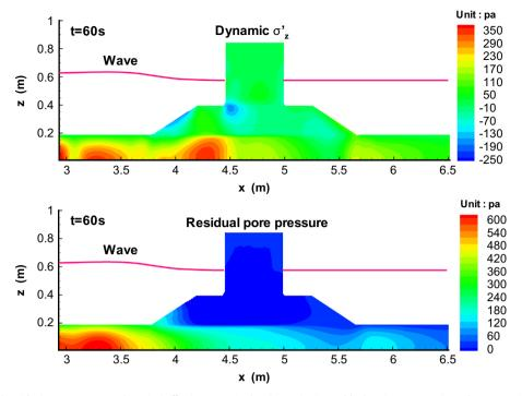
Fig. 16. Wave-induced residual pore pressure and vertical effective stress in the elasto-plastic sand bed at time t=60 s. (Noted: compressive stress is negative.)
