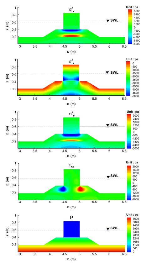
**Fig. 5.** Distribution of effective stresses  $\sigma'_{\chi}$ ,  $\sigma'_{\chi}$  and  $\tau_{\chi z}$ , and pore pressure *p* in the consolidation status.
