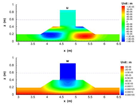
**Fig. 6.** Distribution of horizontal and vertical displacement *u*, *w* in the consolidation status.
