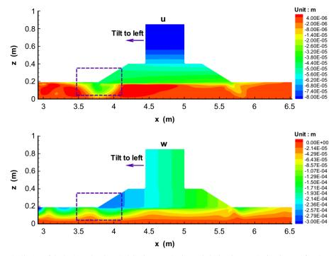
Fig. 18. Distribution of the horizontal and vertical displacement in the sandy bed and composite breakwater after time t/T=50.
