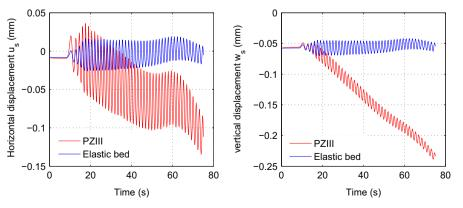
**Fig. 10.** Horizontal and vertical displacement of typical point (x=4.45 m, z=0.85 m) on the breakwater.
