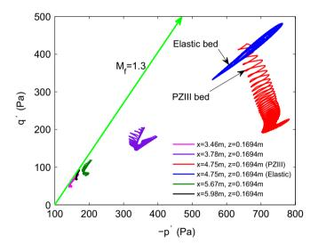
Fig. 17. Effective stress path at five representative positions in the elasto-plastic loose bed.
