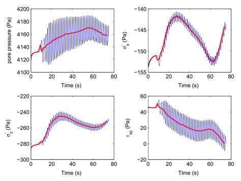
**Fig. 13.** Time history curve of wave-induced pore pressure and effective stresses in the sand bed at C (x=5.67 m, z=0.1694 m), which is under the right foot of the rubble mound.
