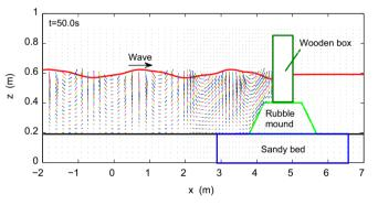
**Fig. 7.** Velocity field of fluid motion in front of breakwater and in porous seabed at t=50 s.
