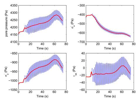
**Fig. 12.** Time history curve of wave-induced pore pressure and effective stresses in the sand bed at B (x=4.725 m, z=0.1694 m), which is under the middle part of the rubble mound.
