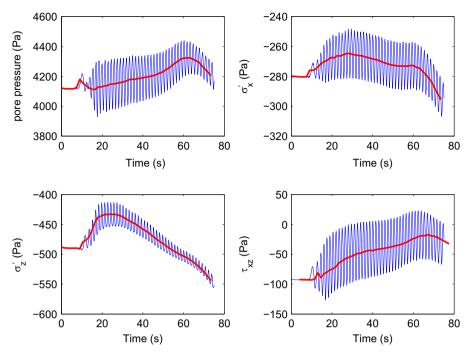
Fig. 11. Time history curve of wave-induced pore pressure and effective stresses in the sand bed at A (x=3.78 m, z=0.1694 m), which is under the left foot of the rubble mound.
