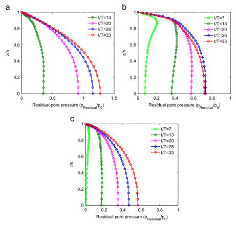
Fig. 15. Distribution of wave-induced residual pore pressure along depth at three different positions in the elasto-plastic sand bed.
