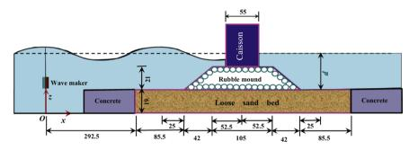
Fig. 2. Set-up and dimension of computational domain similar with the wave flume test conducted by Mostafa et al. (1999).
