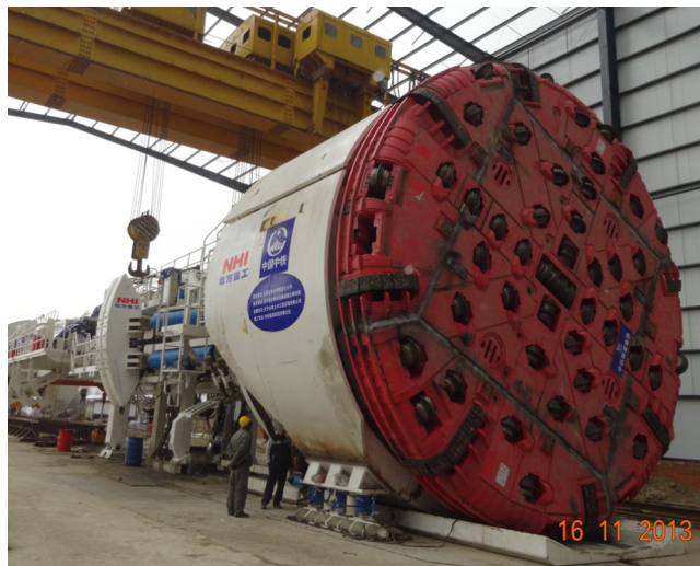
Fig. 2. Gripper TBM employed in this study.
