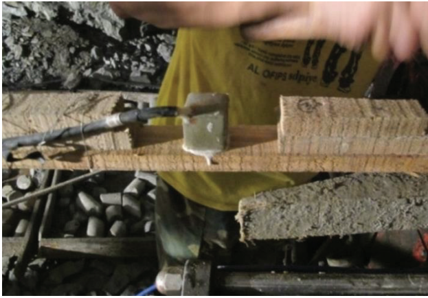
(a) Bonding strain blocks on wood sticks
