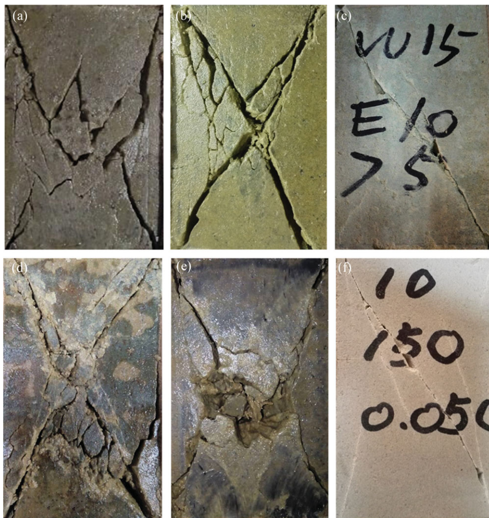
Figure 4. Typical crack extension and failure modes of fluid-saturated sandstones: (a) injected CO 2 ; (b) injected N 2 ; (c) injected H 2 O; (d) near CO 2 injection side under CO 2 -H 2 O biphasic conditions; (e) near H 2 O injection side under CO 2 -H 2 O biphasic conditions; (f) dry.
